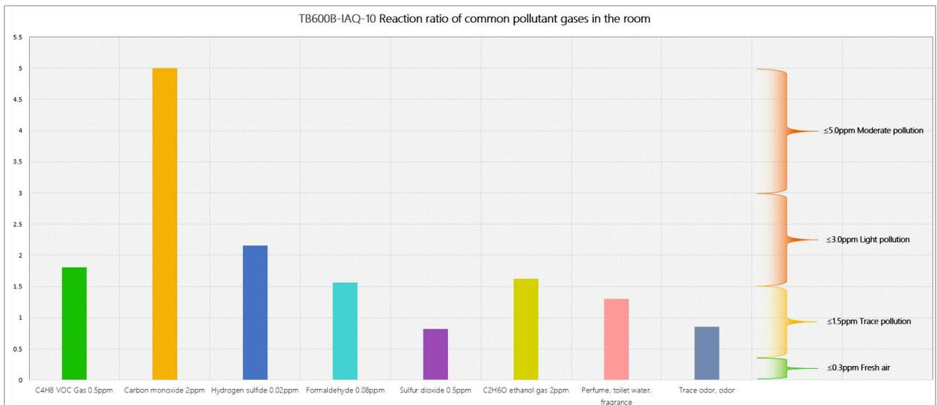
The IAQ air quality sensor module's main indoor pollutants are: TVOC gas, formaldehyde, methanol, toluene, sulfur dioxide SO<sub>2</sub>, carbon monoxide CO, hydrogen sulfide H<sub>2</sub>S, methyl mercaptan CH<sub>4</sub>S, hundreds of toxic gases such as CH hydrocarbons and SO<sub>x</sub> sulfur oxides have good reaction characteristics.
