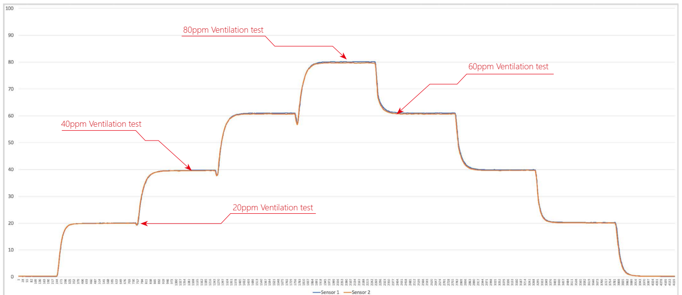
Test result: 0- 50ppm linear error <± 3%; 50- 100ppm linear error <± 5%;
